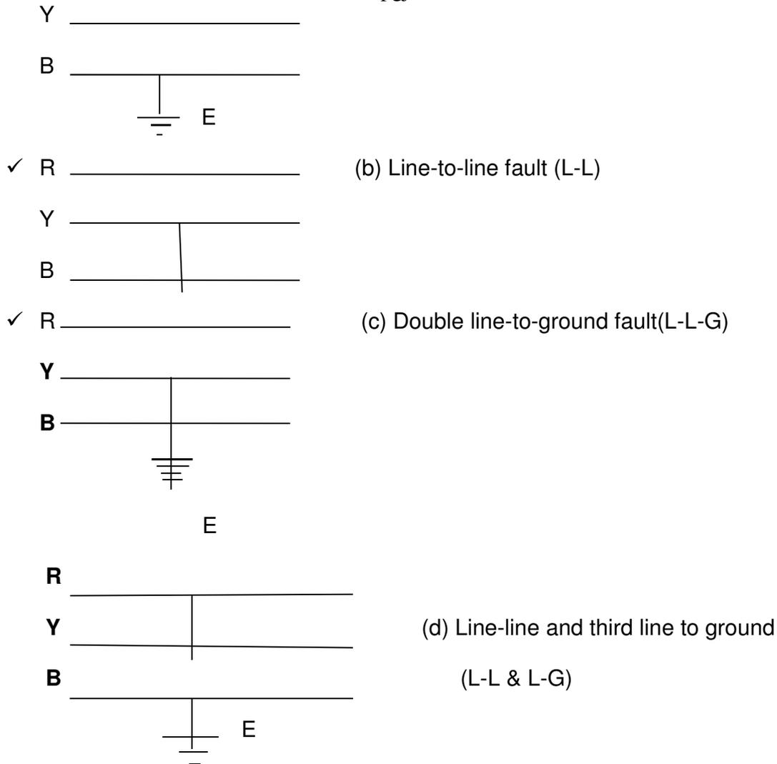
**Fig.1: Different forms of unbalanced faults.**
