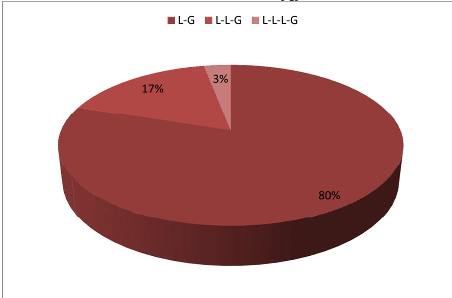
**Fig.7: Chart showing the percentage occurrence of the various earth faults.**
