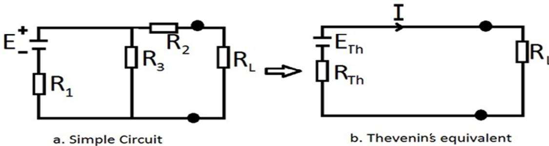
Fig.3: Thevenin's equivalent (b) of a simple circuit (a).
