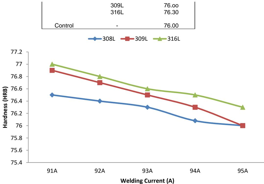
Figure1. Effect of Welding Current on Hardness of Welded Joint
