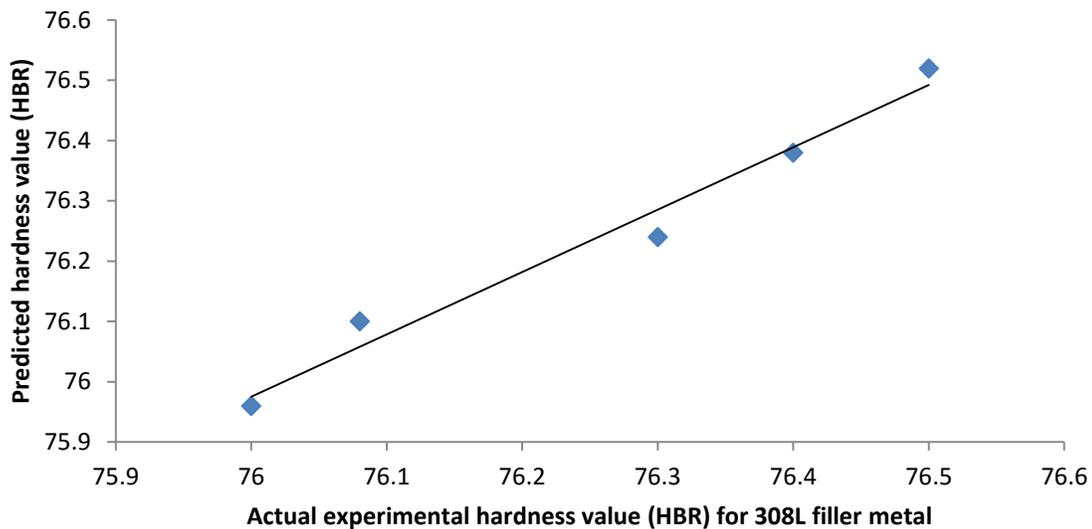
**Figure 4. Scatter diagram for 308L filler metal**
