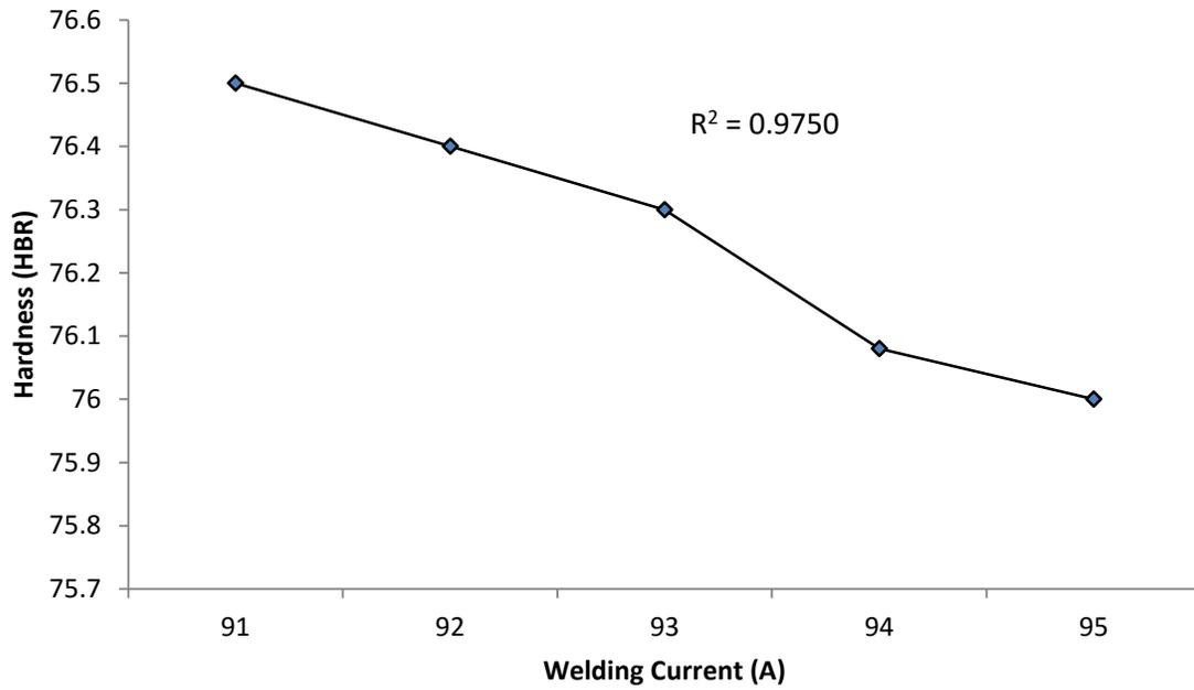
**Figure 2. Interaction between actual experimental hardness value and welding current for 308L filler metal**
