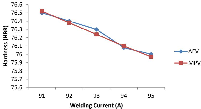
**Figure 1. Interaction between hardness and welding current for 308L filler metal**
